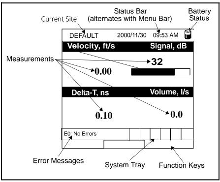
Figure 6: PT878 Screen in Operate Mode
